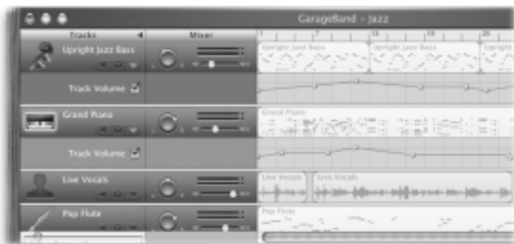
Figure 4-7: Once you've exposed the Track Volume strip, you can click on the colored line—a graph of the track volume—to insert a handle, which you can drag to make the volume rise and fall over time. (Make sure that the Track Volume checkbox is turned on if you want to hear the effect.)
